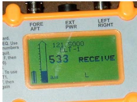
Figure 4. L-Per® Operating Screen in the Receive Mode.
