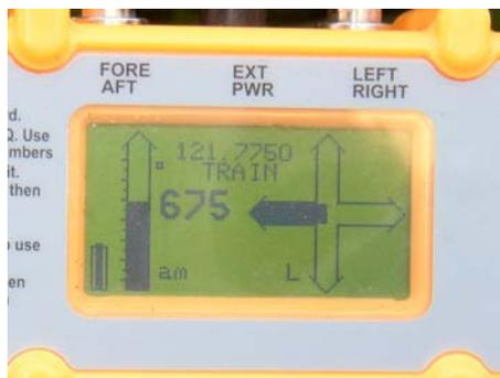
Figure 3. L-Per® Operating Screen in the DF Mode.
